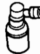
PCV VALVE EV 141 REPLACE AT RECOMMENDED INTERVAL (NATURALLY ASPIRATED VALVE SHOWN, TURBO CHARGED VALVE TYPICAL)
