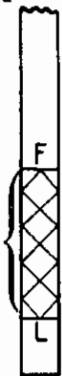
ENGINE OIL DIPSTICK WITH VEHICLE PARKED ON LEVEL GROUND, MAINTAIN OIL LEVEL IN THIS RANGE
